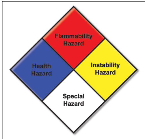
Figure 2: National Fire Protection Rating System (NFPR)
