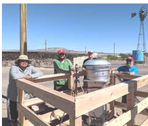
This R2D2-looking machine is a Tisch PM sampler that collects airborne dust for later analyses of metals and other hazardous substances released to the air in each village.
